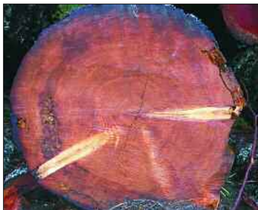
This log would be rejected for the export market due to rot and excessive knot size.
